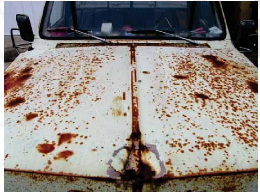
The image is the hood of a truck that has been in a hot climate near the ocean.
