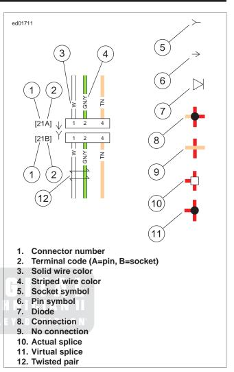
Figure B-1. Connector/Wiring Diagram Symbols
