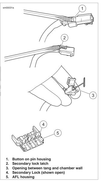
Figure A-27. 480 Metri-Pack Connector: Remove Socket Terminal
