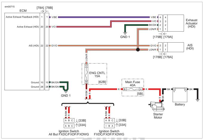
Figure 6-35. Active Exhaust Actuator and AIS Circuit
