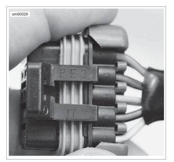
Figure A-25. 280 Metri-Pack Connector (P.E.D.)
