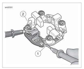
Figure 3-15. Brush Holder Insulation Test
