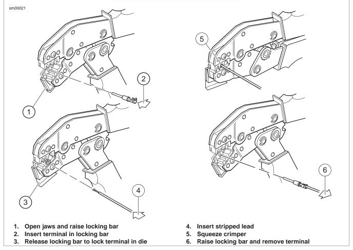
Figure A-17. Crimping a Deutsch Standard Terminal
