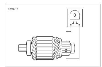
Figure 3-12. Armature Open Test
