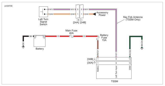
Figure 5-26. Antenna Circuit: TSSM
