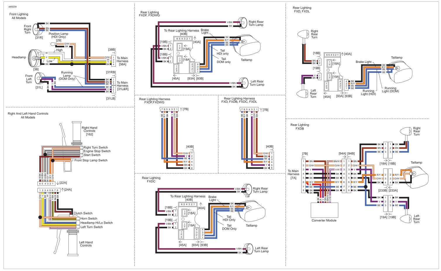
Figure B-16. Lighting, Hand Controls, and Adapter Harnesses: 2010 Dyna
