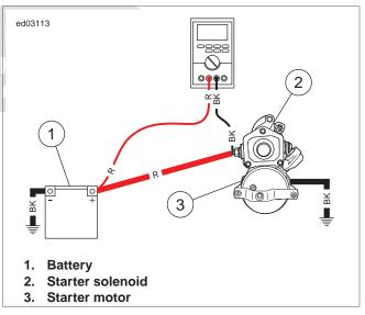
Figure 1-24. To Starter Solenoid Battery Terminal
