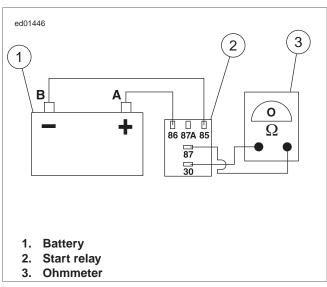
Figure 1-29. Five Terminal Relay Test
