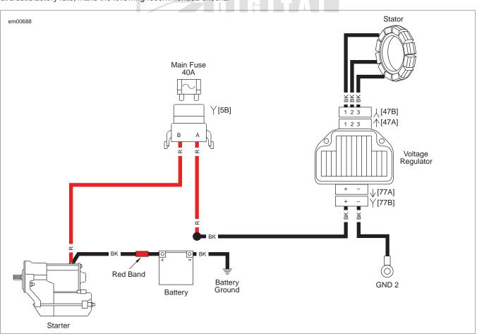
Figure 3-16. Charging System Circuit
