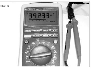
Figure 3-21. Check Stator AC Voltage Output (Typical)
