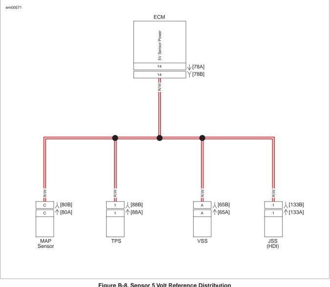
Figure B-8. Sensor 5 Volt Reference Distribution
