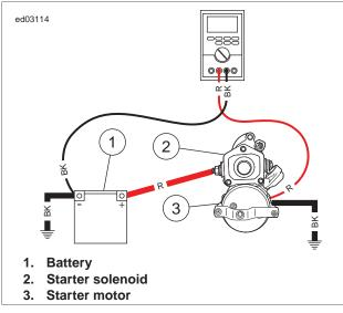
Figure 1-25. Starter Ground Circuit
