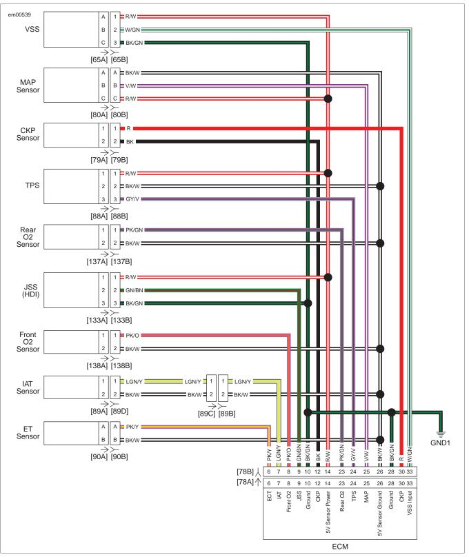
Figure 6-4. Sensor Circuit
