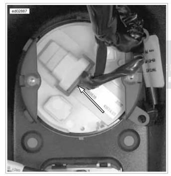
Figure 3-23. Speedometer Connector [39]
