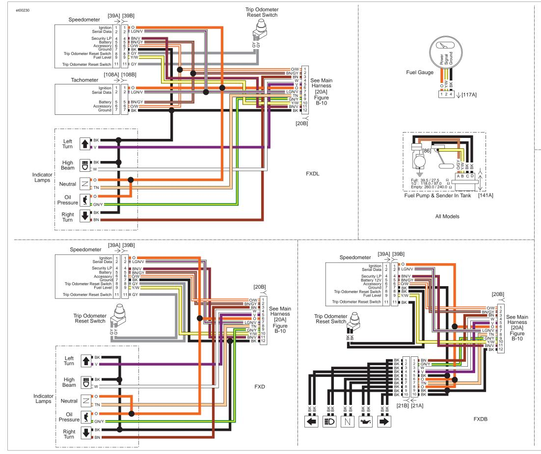
Figure B-13. Instruments and Indicators: 2010 Dyna
