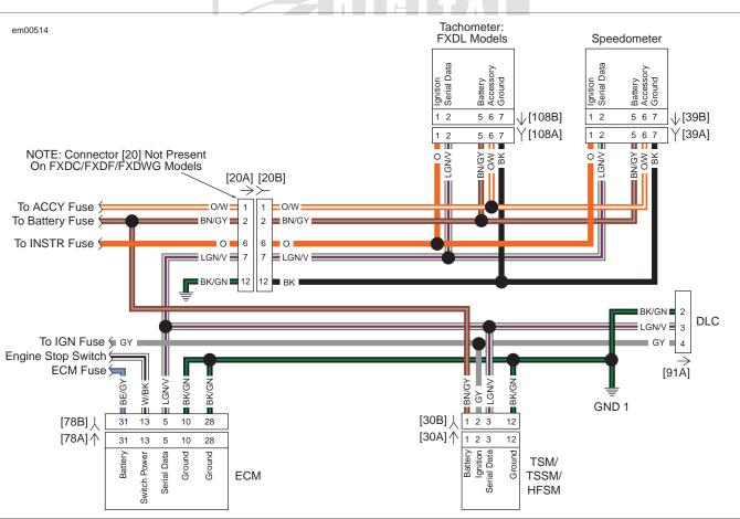
Figure 2-8. Serial Data Circuit
