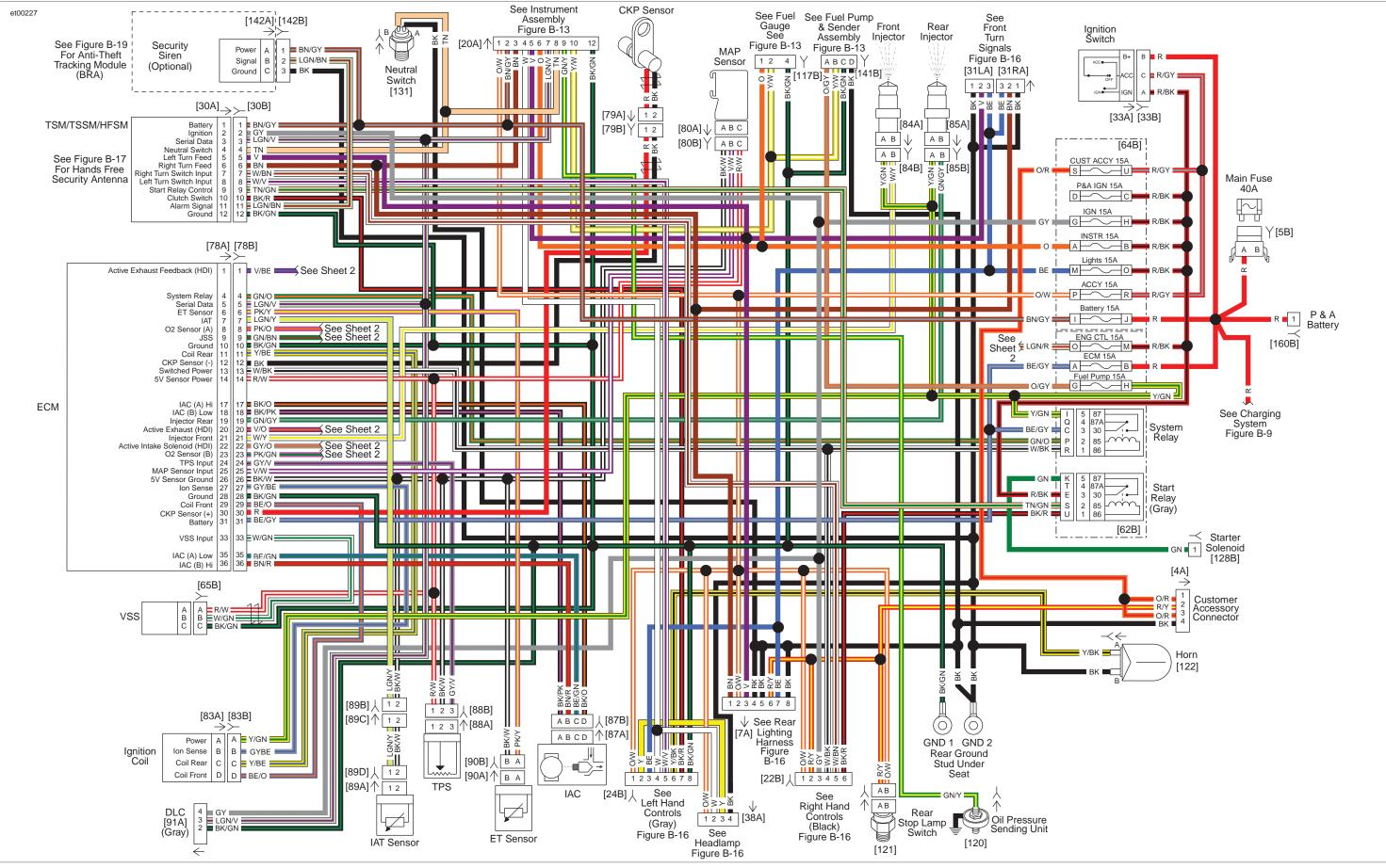
Figure B-10. Main Harness (1 of 2): 2010 Dyna (FXD, FXDB, and FXDL)
