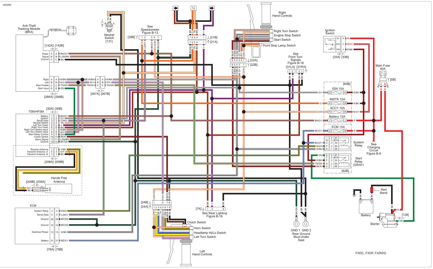
Figure B-20. Security Circuit, Anti-Theft Tracking Module (BRA): 2010 Dyna (FXDC, FXDF, and FXDWG)
