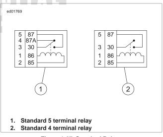
Figure 1-27. Standard Relays
