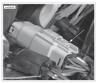
Figure A-33. Molex Connector: Latch
