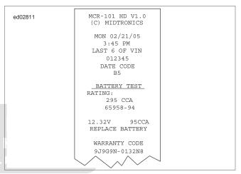
Figure 3-1. Battery Test Results Printout
