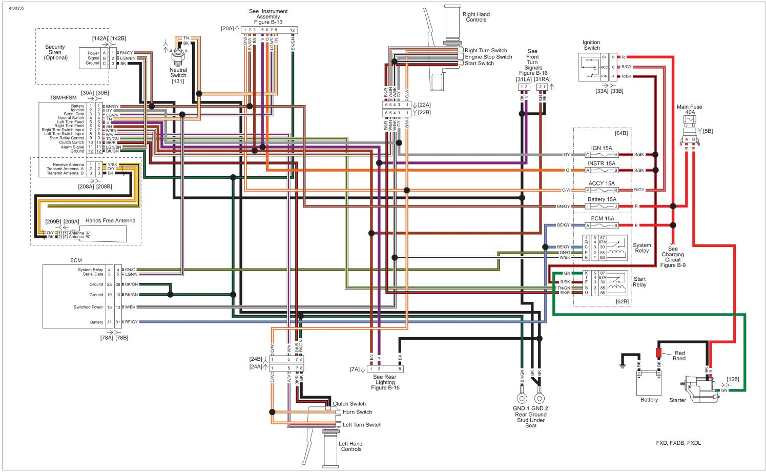
Figure B-17. Security Circuit: 2010 Dyna (FXD, FXDB, and FXDL)
