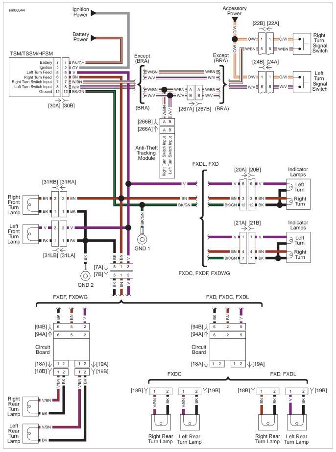
Figure 5-19. Turn Signal Circuit (Except FXDB)
