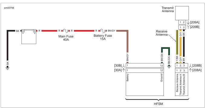
Figure 5-31. Antenna Circuit: HFSM
