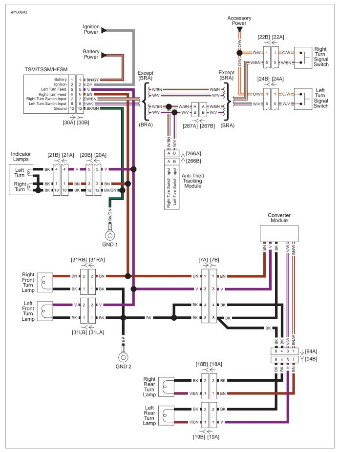
Figure 5-18. Turn Signal Circuit (FXDB)
