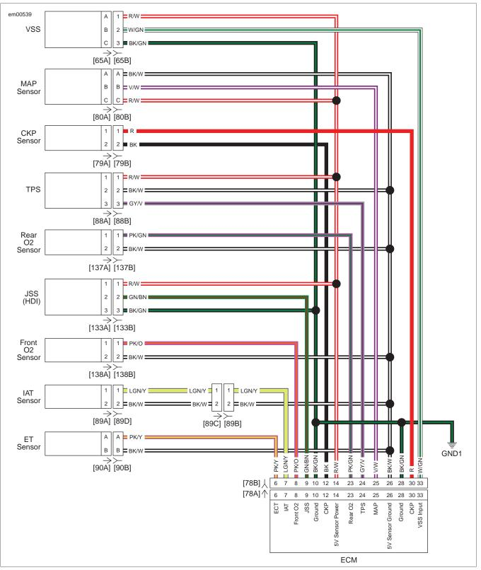
Figure 6-37. Sensor Circuit
