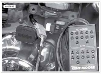
Figure 1-20. Breakout Box: TSM/HFSM
