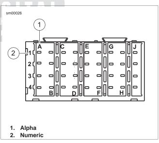
Figure A-22. Fuse Block: Coordinates (typical)
