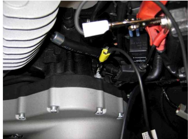
Pull top of left side cover down. Cover is hinged at the bottom.
