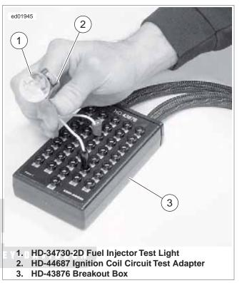
Figure 1-16. Fuel Injector Test Light
