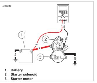
Figure 1-23. To Starter Solenoid Starter Terminal
