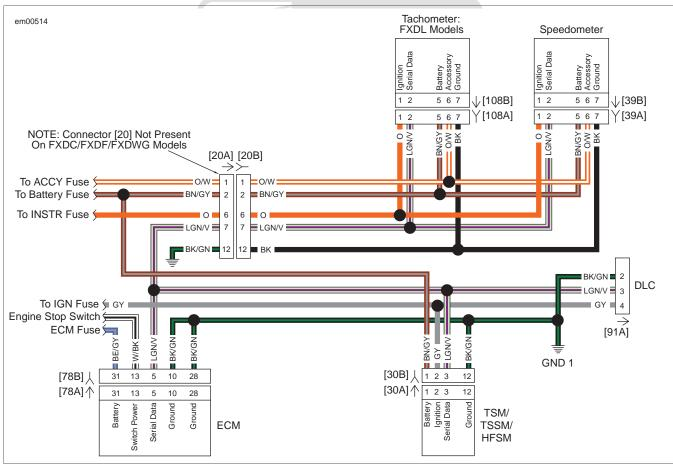
Figure 6-26. ECM and TSM/TSSM/HFSM Circuit
