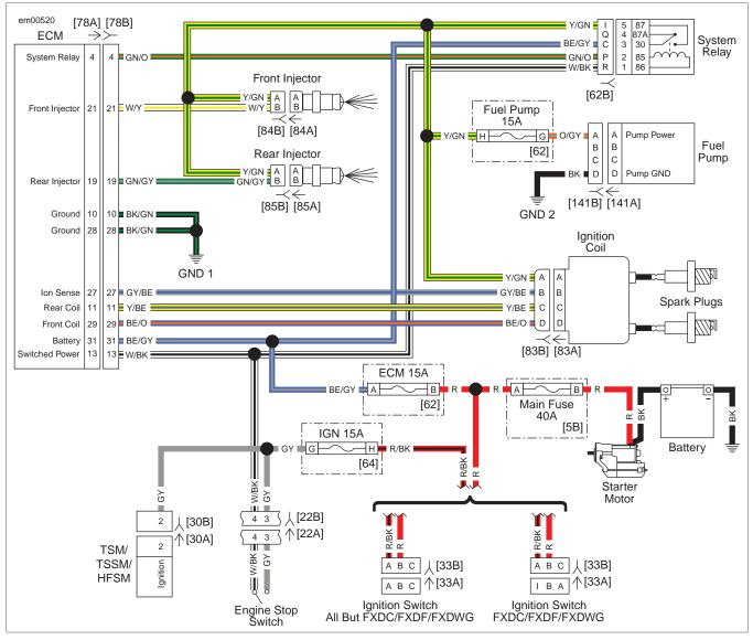
Figure 6-31. Ignition Circuit
