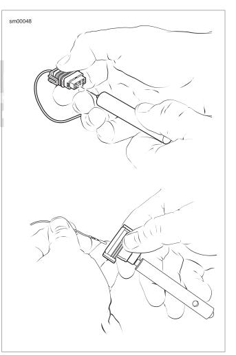
Figure A-42. Packard Micro 64 Connector: Insert Tool and Remove Terminal
