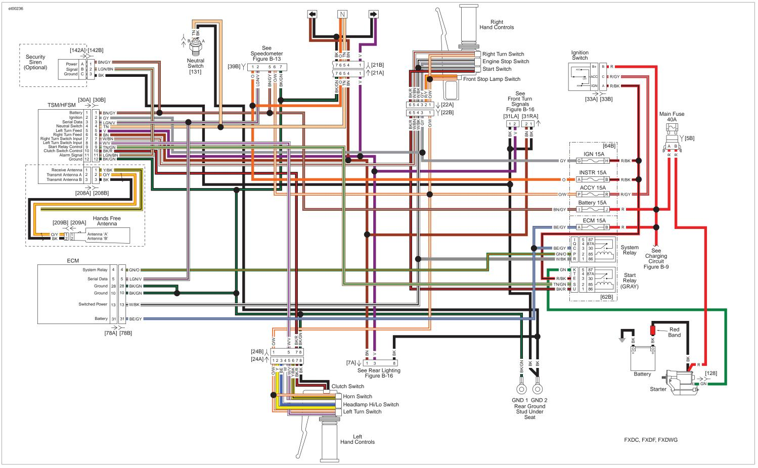
Figure B-18. Security Circuit: 2010 Dyna (FXDC, FXDF, and FXDWG)
