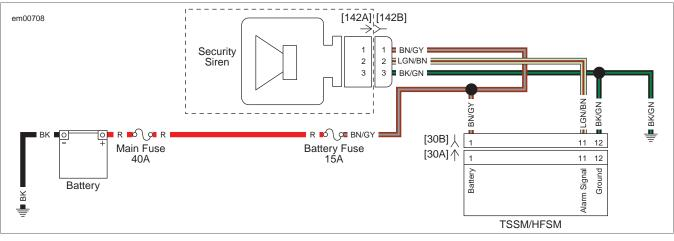
Figure 5-28. Smart Siren Circuit
