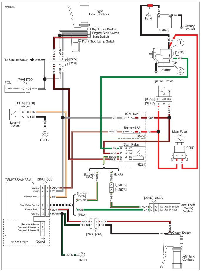
Figure 3-4. Starting Circuit
