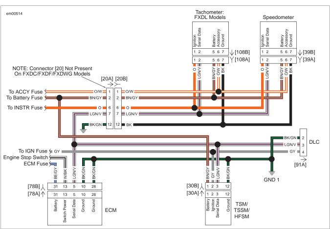
Figure 2-9. Serial Data Circuit
