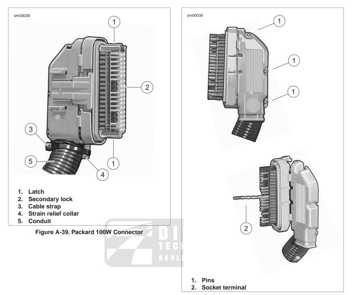
Figure A-40. Packard 100W Connector: Separate Halves of Socket Housing
