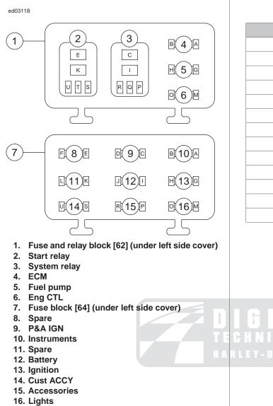
Figure B-2. Fuse Block and Socket Terminals
