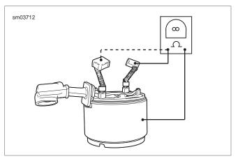
Figure 3-13. Grounded Field Test
