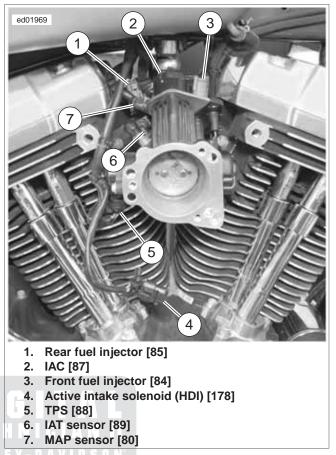
Figure 6-13. Between Cylinders Right Side
