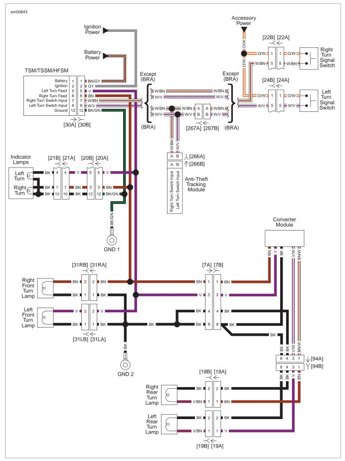
Figure 5-8. Turn Signal Circuit (FXDB)
