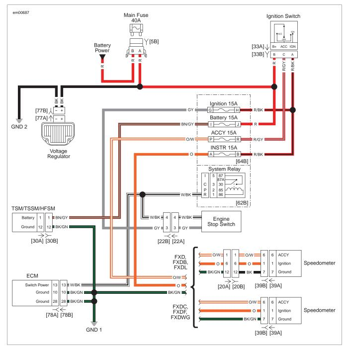
Figure 3-22. High and Low Voltage Sensors
