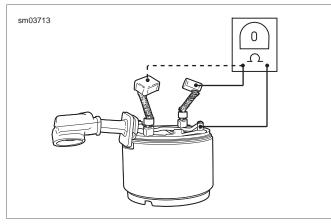
Figure 3-14. Open Field Test
