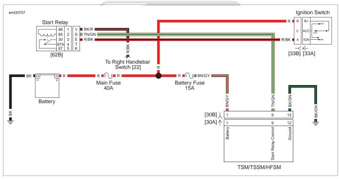
Figure 5-30. Starter TSM/TSSM/HFSM Circuit
