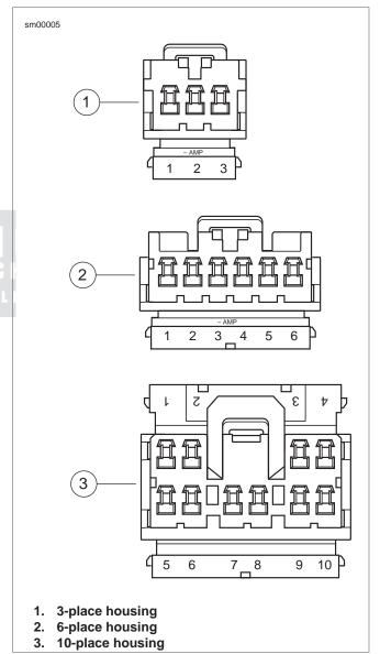
Figure A-3. AMP Multilock Connector: Cavity Numbers on Secondary Locks (Socket Housings Shown)
