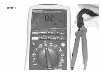
Figure 3-20. Check for Stator Resistance (Typical)
