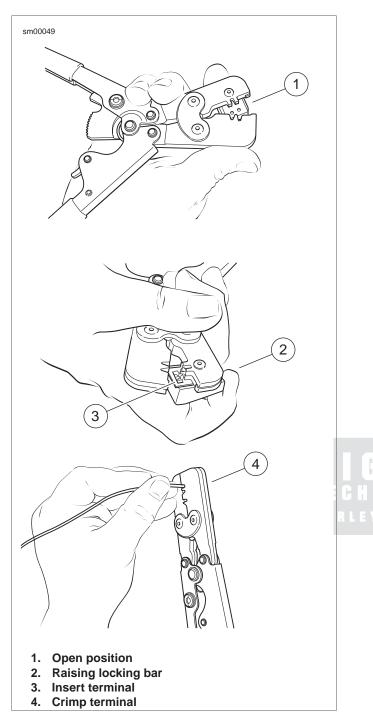
Figure A-45. Packard Micro 64 Connector: Terminal in Crimper
