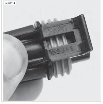
Figure A-8. Delphi Connector: Socket Housing Latch
