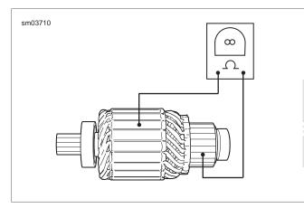
Figure 3-11. Grounded Armature Test
