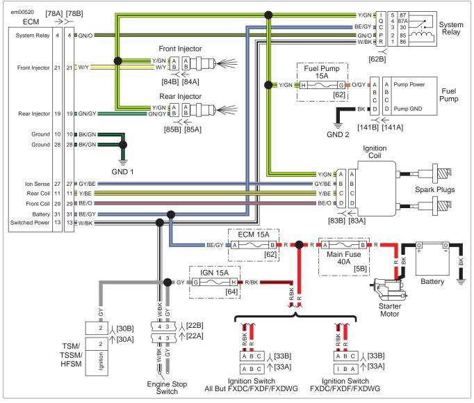
Figure 6-40. Ignition Circuit
