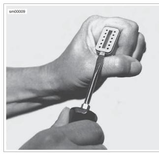
Figure A-12. Deutsch Connector: Remove Secondary Locking Wedge
