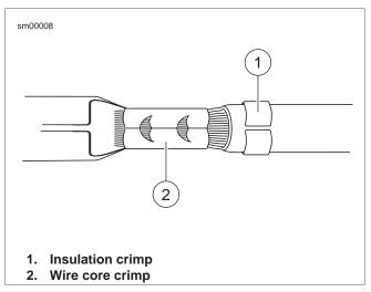
Figure A-7. AMP Multilock Connector: Terminal Crimp
