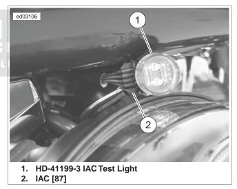
Figure 6-19. IAC Test Light (Part No. HD-41199-3)
