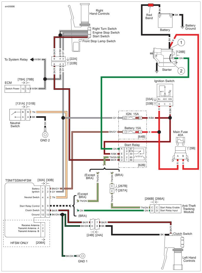
Figure 5-33. Starting Circuit
