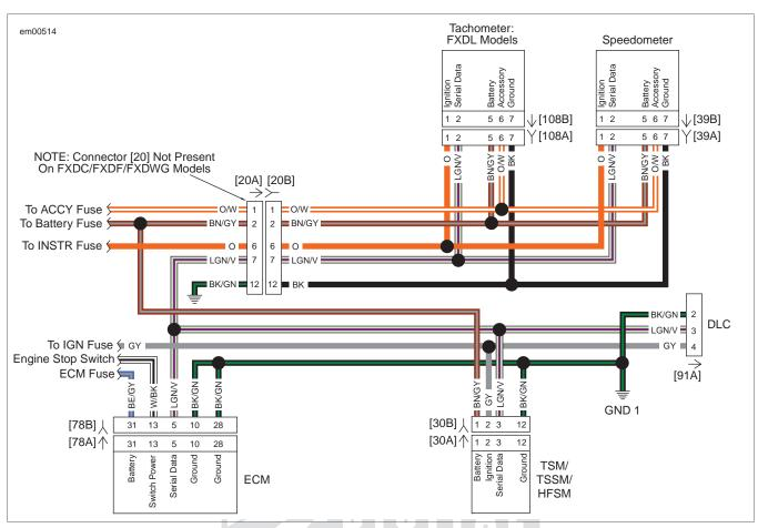
Figure 4-6. Instruments Power Circuit Diagram
