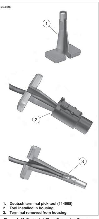
Figure A-10. Deutsch 1-Place Connector: Remove Socket/Pin Housing
