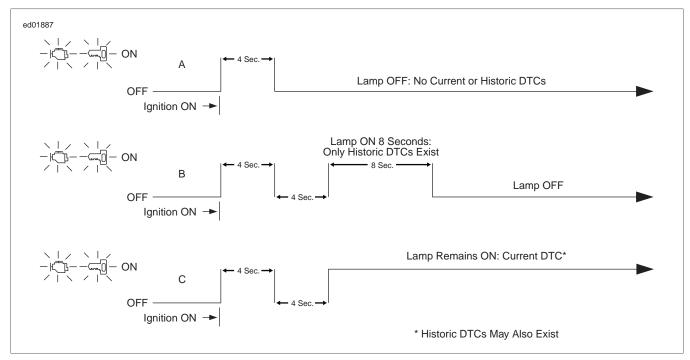
Figure 2-1. Check Engine Lamp and Security Lamp Operation
