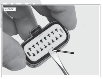
Figure A-34. Molex Connector: Secondary Lock Pry Slot (Socket Housing)
