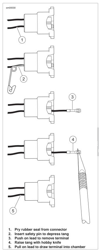
Figure A-26. 280 Metri-Pack Connector: Remove/Install Socket Terminal
