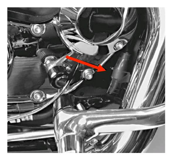
**NOTE:** Follow the two wires <u>coming out</u> of the lower right side of the engine. These are from the stator.
