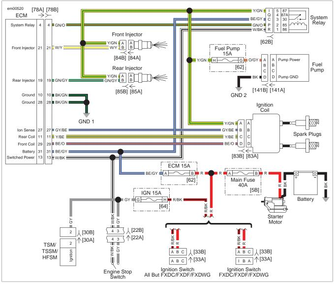
Figure 6-47. Ignition Circuit
