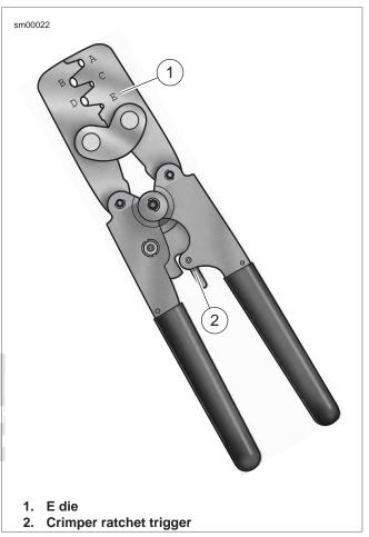
Figure A-18. Packard Terminal Crimper (HD-38125-7)
