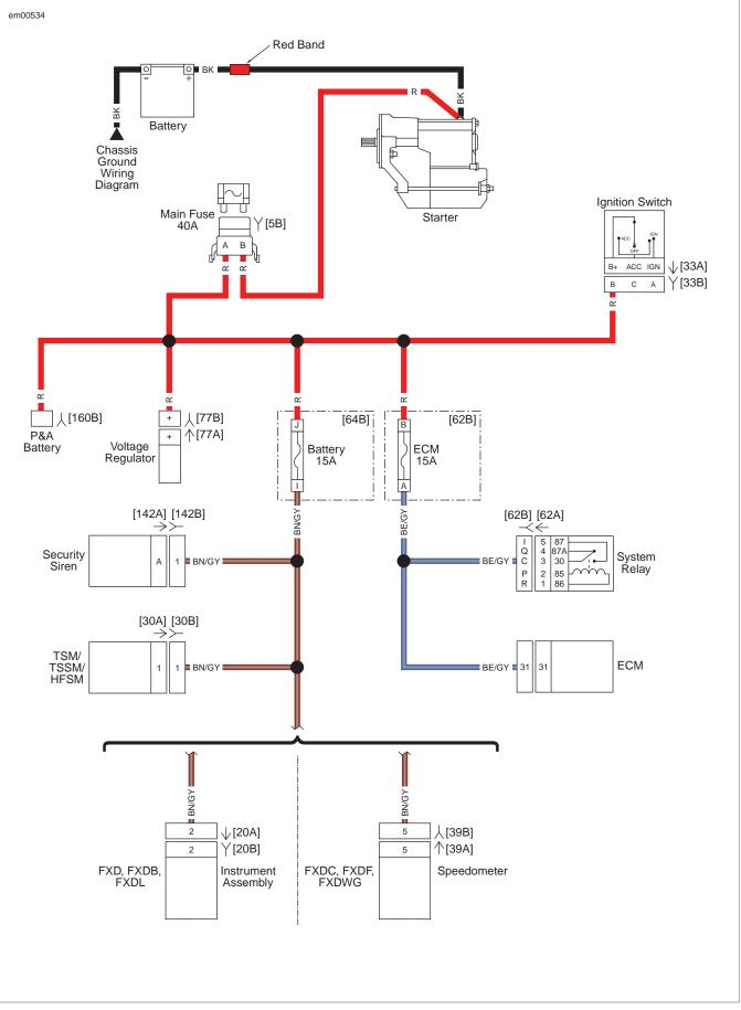
Figure 2-2. Battery Power
