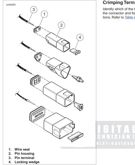
Figure A-16. Deutsch Connector: 2, 3, 4 and 12-Place Pin Housings
