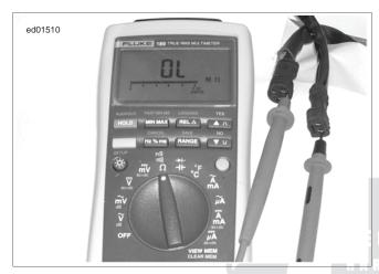
Figure 3-19. Test for Grounded Stator (Typical)
