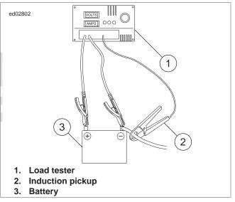
Figure 3-18. Check Current Draw (Ignition Switch On)
