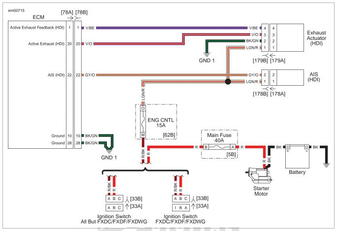
Figure 6-24. Active Exhaust Actuator and AIS Circuit
