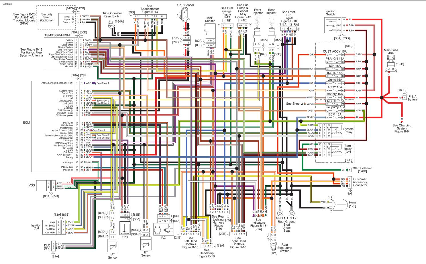
Figure B-11. Main Harness (1 of 2): 2010 Dyna (FXDC, FXDF, and FXDWG)
