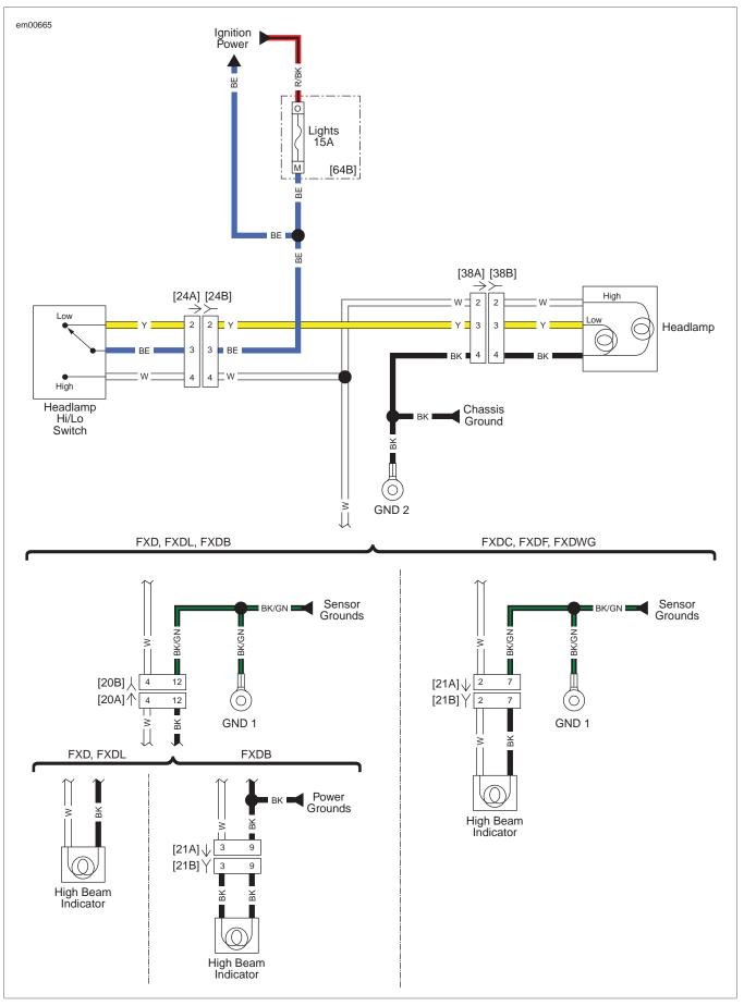
Figure 5-11. Headlamp and Running Lamps
