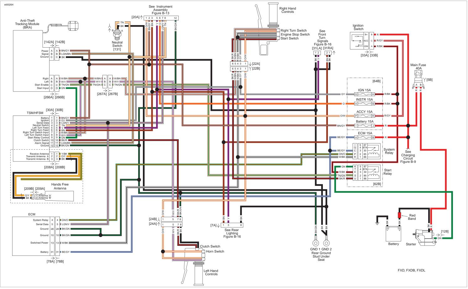
Figure B-19. Security Circuit, Anti-Theft Tracking Module (BRA): 2010 Dyna (FXD, FXDB, and FXDL)
